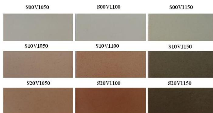
**Figure 2.** Macro images of non-additive and vermiculite additive sanitaryware samples.
