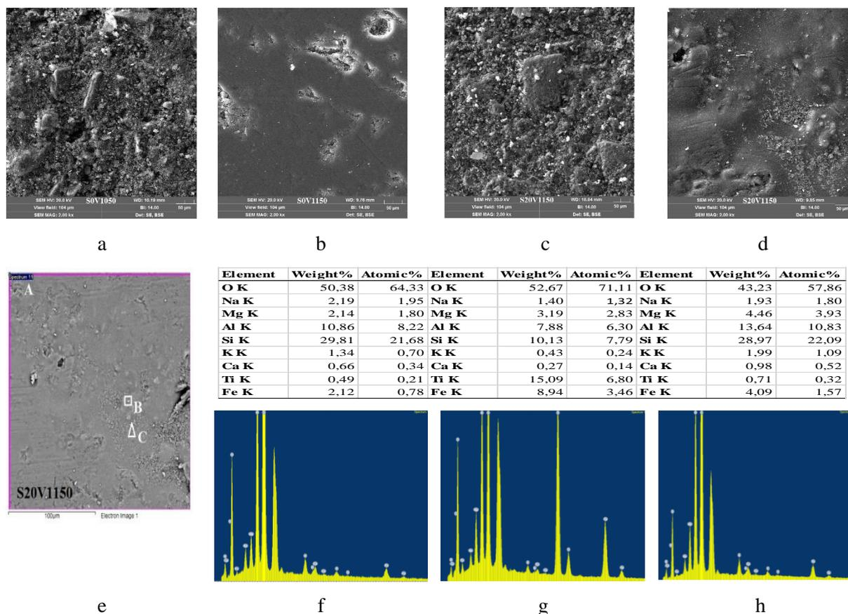
**Figure 4.** SEM images of sintered samples at 1050 °C and 1150 °C. a) S0V1050 b) S0V1150 c) S20V1050 d) S20V1150. EDX analyses %20 vermiculite additive sanitaryware samples sintered 1150°C. e) image of EDS area and f) area of A EDS g) B point EDS and h) C point EDS.
