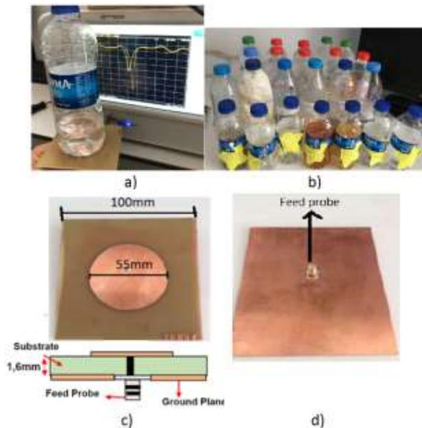
Fig.1. a) Measurement system used in this study b) Samples c) The geometry of the antenna and front view of the antenna d) Back view of the antenna.
