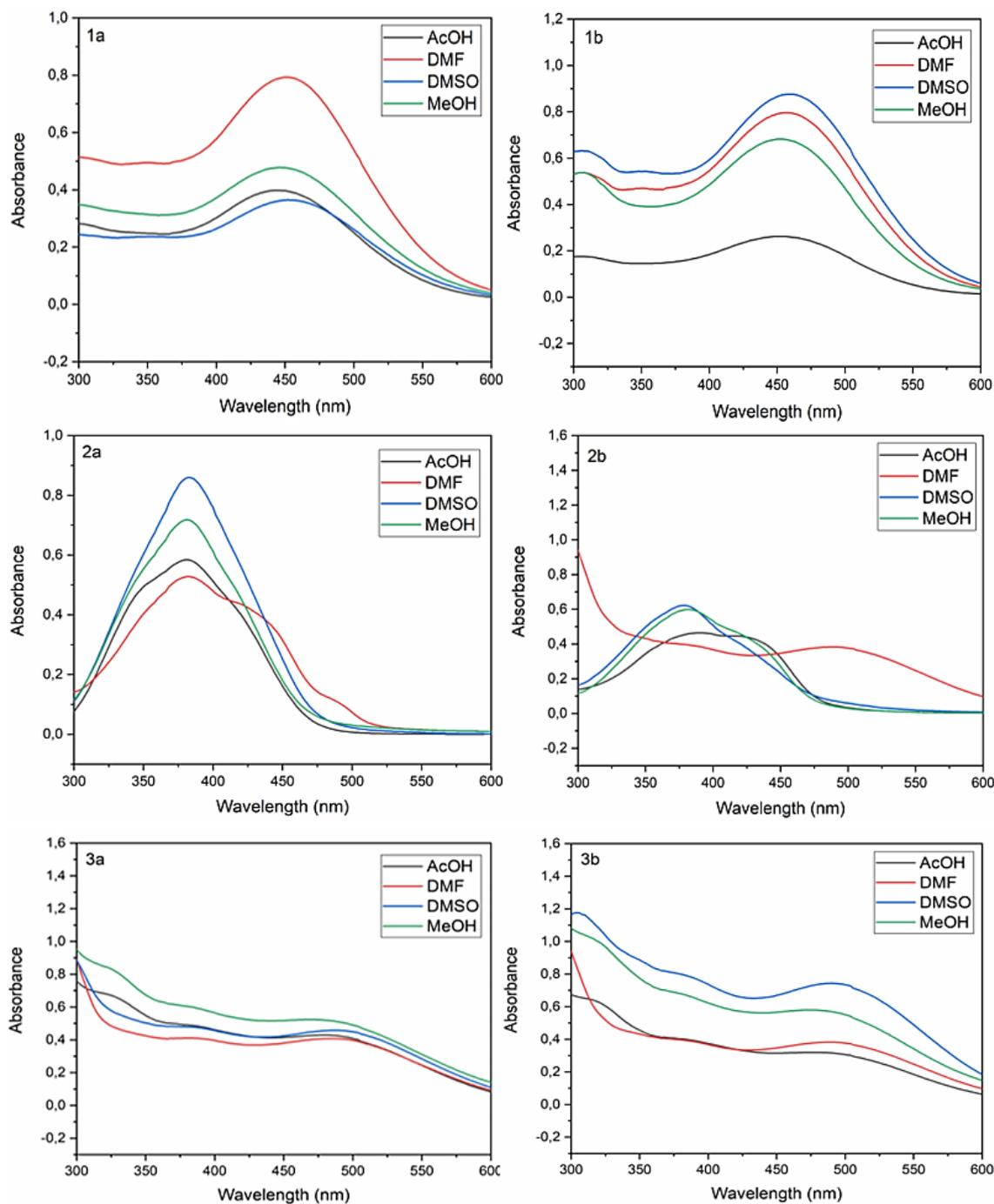
**Figure 3.** Absorption spectra of synthesized compounds in various solvents
