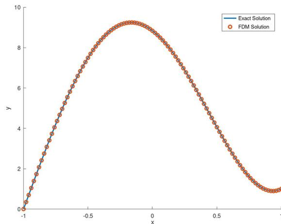
**Figure 3.2:** Comparison of the FDM-solution with the exact solution for  $N=100$ .
